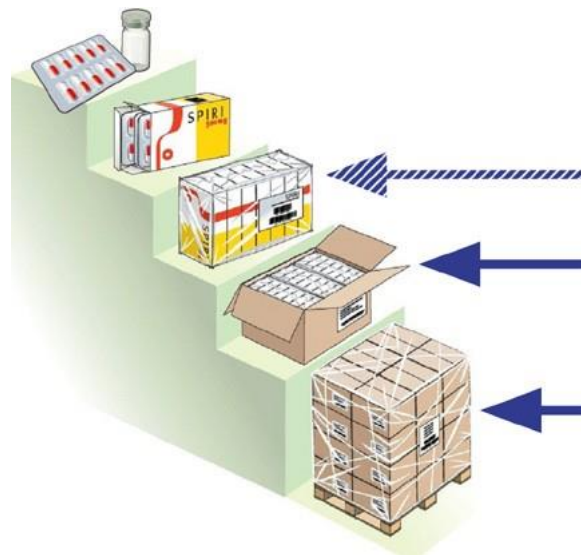
Figure 1: Packing cascade (as in ISO/DTS 16791-2012)
