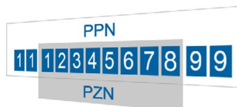
For the purpose of transferring the PPN by Matrix Code and RFID, the international distinct Data Identifier (DI) „9N“ (according the ISO/IEC 15418 rules) has been assigned to the PPN. The complete methodology for generating the PPN and its check-digit is described in the following document: 'Technical Specification – PPN'
